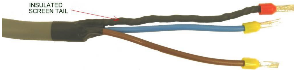
Figure 33 Power cable Screen Tail Insulation.
