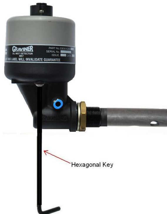
Figure 121 Base Fixing Screw Removal
