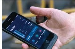
The GLC X controller is Bluetooth enabled, so maintenance crews and operators can quickly monitor a wide range of lubrication metrics, including levels, pressure, configurations and more.
