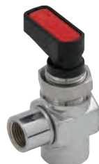
Haaks - L-boring - BSP female - paneelmontage
