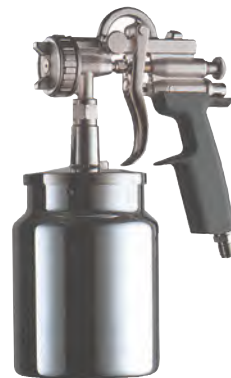
Type UR-Plus-1000 - 3-4.5 bar - aluminium 1000cc onderbeker
