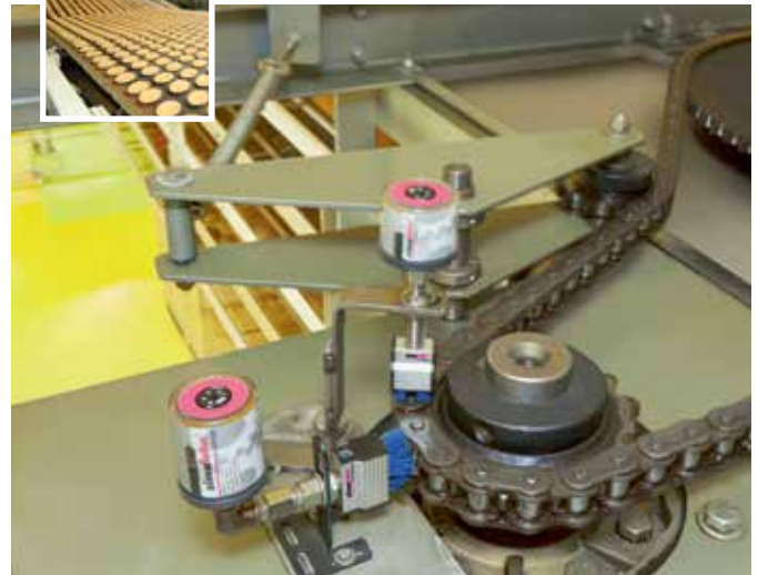
The drive chain of a transport belt, which allows rolls to cool, is cleaned with special blue brushes and lubricated with 2 simalube SL18 in 30 and 60 ml sizes.
